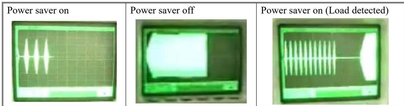
Note: The minimum power of load to take inverter out of sleep mode (Power Saver On) is 25 Watts.
