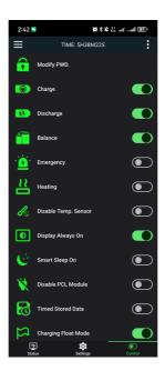
Through BMS control, the protection board can be charged, discharged, balanced, switched on and off, and emergency switched on.
